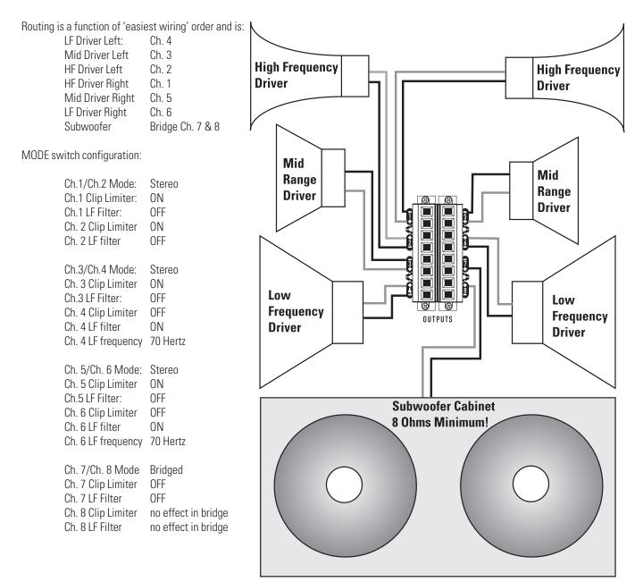
Channels 1 through 6 are configured for 'stereo' mode because all channels are completely separate from one another. Channels 7 and 8 are bridged to combine their power to drive the subwoofer (sub's are the most inefficient driver and therefore require the largest portion of the system power).
